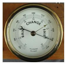
A **barometer** measures atmospheric pressure.
