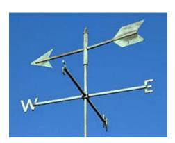
A **wind vane** is used to show the direction of the wind.
