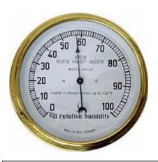
A **hygrometer** measures humidity or the amount of water vapor in the air.
