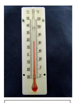
**Thermometers** measure the temperature of the surrounding air in degrees Fahrenheit and/or Celsius.
