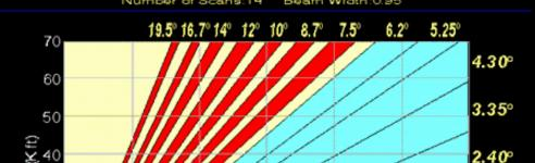
A 7,500 ft. circulation is easily resolved at 20 - 30 nautical miles, but the same circulation cannot be seen by the radar 100 nautical miles away.
