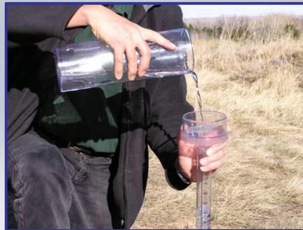
*Pour the remaining water into the funnel and measure the inner tube.*
