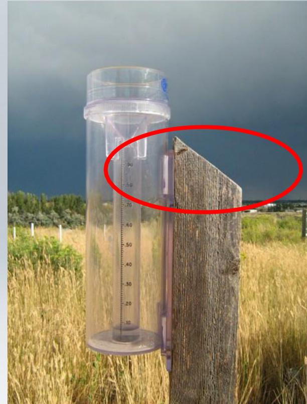
Bevel the top of the post to reduce rain splashing into the gauge
