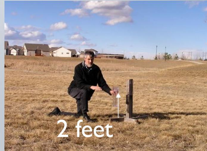
In developed areas place the gauge top approx. 5 feet off the ground
