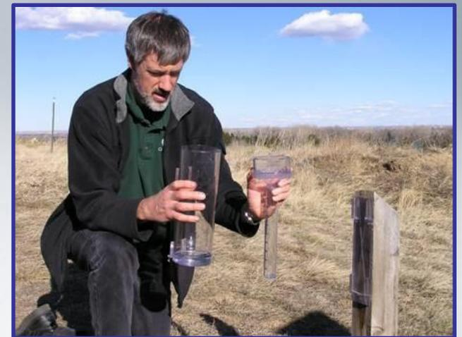
*Continue until all of the water has been measured. Make sure you keep track of your measurements along the way.*
