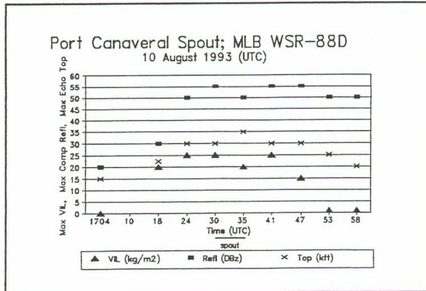
Fig. 11. Radar observed parameters for the spout cell. The estimated time and duration of the spout is indicated with a bold line below the time axis.
