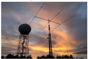
KMLB WSR-88D Radar and CL-33 Rotatable Beam
