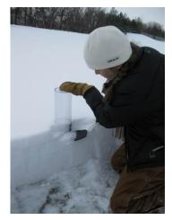
container like a bucket or trash can. Then take the empty rain gauge back to the same location, turn it upside down and push it back into the snow to gather the remainder of the snow down to the ground. Dump the additional snow into the bucket with the previous sample, so all of the snow can be melted down and measured.
