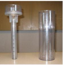
Placement of the **rain gauge** is critical for the most representative measurements possible.
