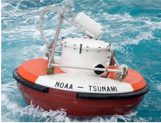
Figure 7. DART system buoy
