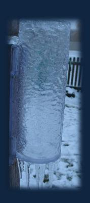
Melt and measure the moisture accumulated inside of the rain gauge in exactly the same way as snowfall water content
