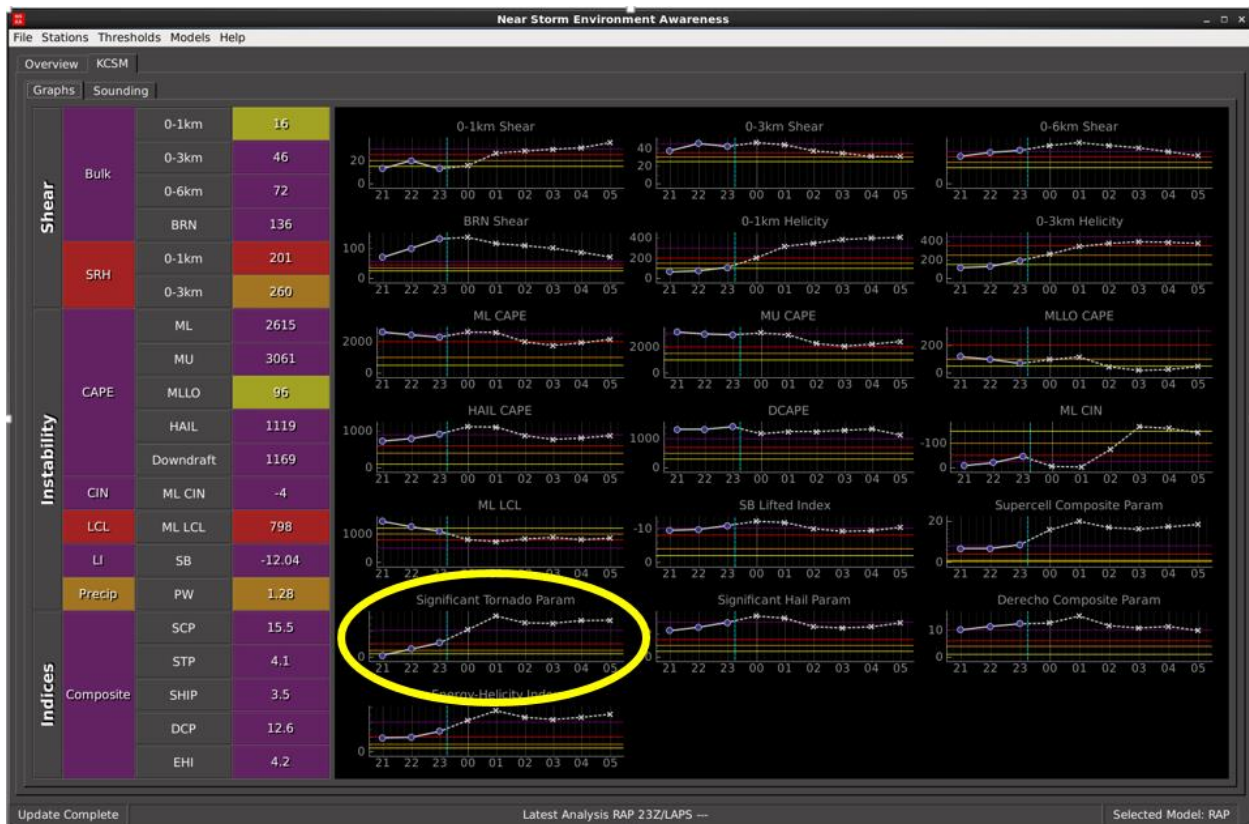
Figure 4 - NSEA Application Time Series Graphs, plotted for all severe weather parameters at Clinton-Sherman Airport, OK (CSM), on 8 MAY 2016. Base time is 2300 UTC, denoted by blue, vertical dashed line. Previous two hours of observed information are plotted to the left of the current time and presented with a blue fill. Ensuring six hourly forecasts, based on the RAP13, are plotted to the right and presented with a white fill. Trends for the Significant Tornado Parameter are highlighted in the graph within the yellow oval.
