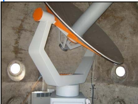
Left: Tracking Antenna as seen from inside the dome.
