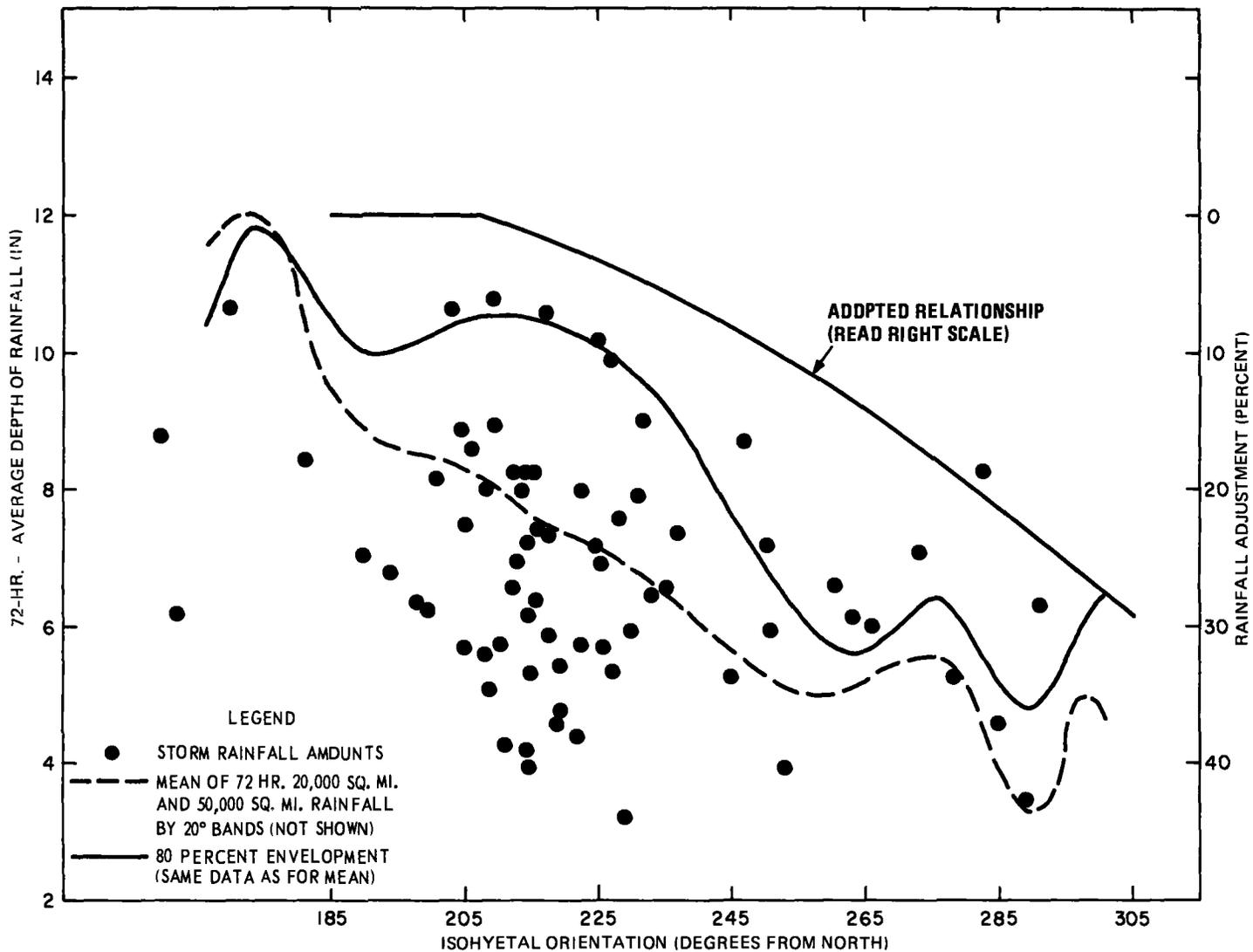
Figure 5-6.--72-hr rainfall versus orientation of major axis of isohyetal pattern. Adopted curve shown. Although only the 20,000-sq-mi 72-hr rain data are shown on this figure, means (of mean and 80% envelopment data) are for both 50,000 and 20,000-sq-mi data.
