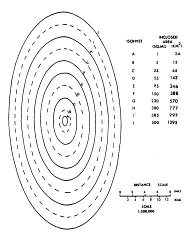
Figure 4.10.--Idealized local-storm isohyetal pattern.
