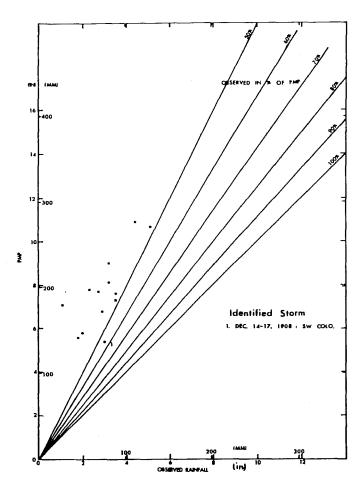
Figure 5.2.--Comparison between observed rainfall depths and general-storm PMP for 5000 mi<sup>2</sup> (12,950 km<sup>2</sup>) 24 hr.
