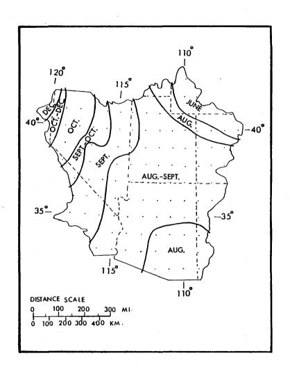
Figure 3.18.--Months of maximum total generalstorm PMP for Southwest States, 10  $\mathrm{mi}^2$  (26  $\mathrm{km}^2$ ) 24 hr.
