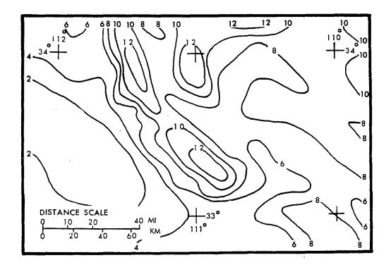
Figure 3.3.--A first approximation to the orographic PMP (inches) for 10  $mi^2$  (26  $km^2$ ) 24 hr in southeast Arizona.
