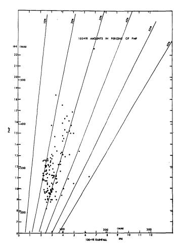
Figure 5.6.--Comparison between 100-yr rainfall (Miller et al. 1973) and PMP. PMP values are the larger of general- or local-storm amounts for 10 mi<sup>2</sup> (26 km<sup>2</sup>) 24 hr at 1° grid points.
