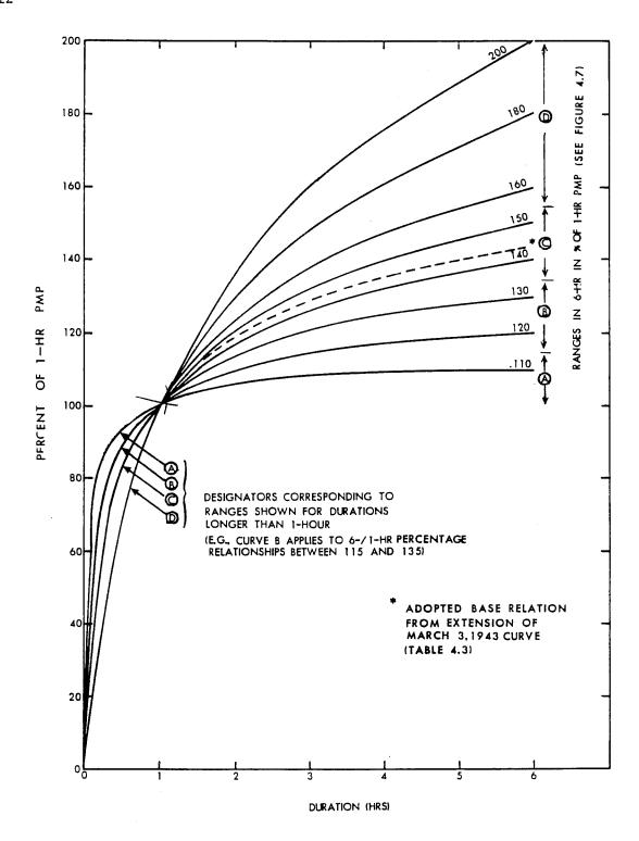
Figure 4.3.--Variable depth-duration curves for 6-hr PMP in the Southwest States and all of California.
