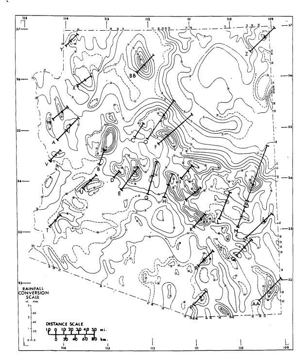
Figure 3.5.--Segments across major ridges in Arizona superimposed on analysis of 100-yr 24-hr precipitation (in tenths of an inch).
