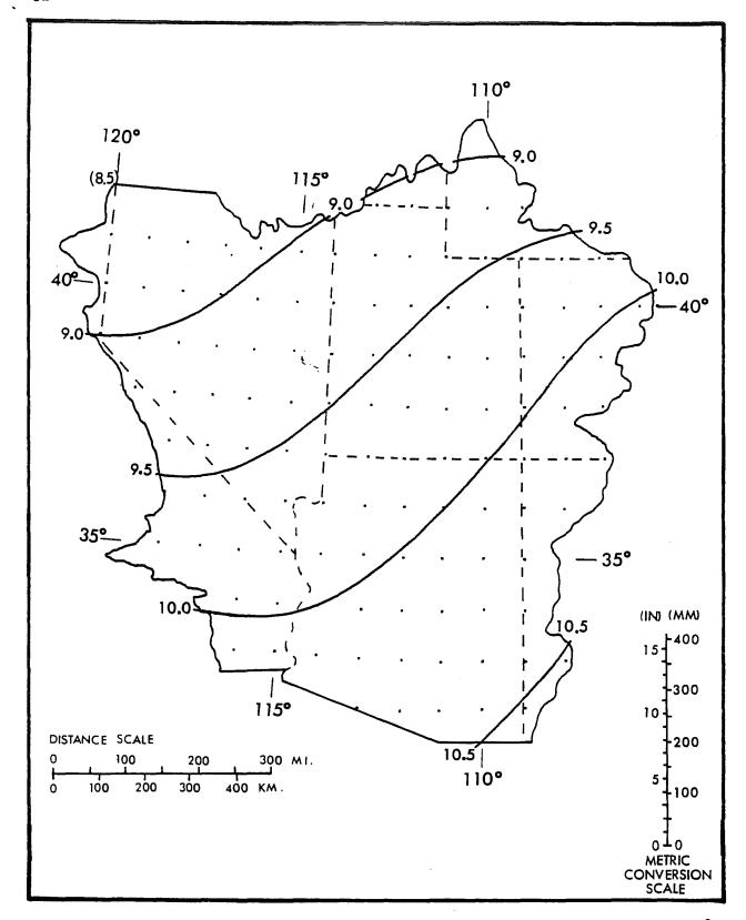
Figure 2.15.--1000-mb (100-kPa) 24-hr convergence PMP (inches) for 10 mi  $^2$  (26 km $^2$ ) for November. Values in parentheses are limiting values and are to facilitate extrapolation beyond the indicated gradient.
