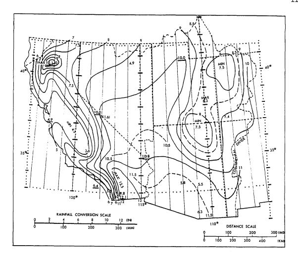
Figure 4.5--Local-storm PMP for 1 mi<sup>2</sup> (2.6 km<sup>2</sup>) 1 hr. Directly applicable for locations between sea level and 5000 ft (1524 m). Elevation adjustment must be applied for locations above 5000 ft.
