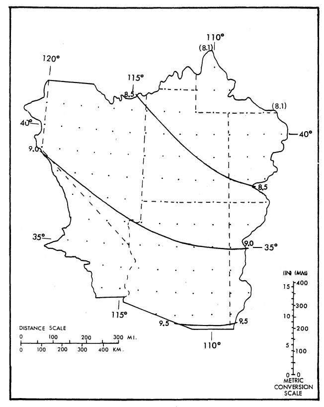
Figure 2.16.--1000-mb (100-kPa) 24-hr convergence PMP (inches) for 10 mi $^2$  (26 km $^2$ ) for December. Values in parentheses are limiting values and are to facilitate extrapolation beyond the indicated gradient.
