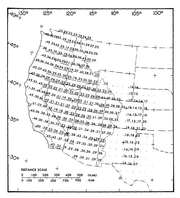
Figure 5.?.--Ratios of 100-yr point rainfall (Miller et al. 1973) to highest PMP for 10 mi<sup>2</sup> (26 km<sup>2</sup>) 24 hr. Underlined ratios are points where 6-hr local-storm PMP controls. East of 105th meridian PMP taken from eastern states study (Schreiner and Riedel 1978).
