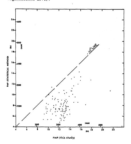
5.9.--Comparison between statistical PMP (Hershfield 1965) and the highest PMP for 10 mi<sup>2</sup> (26 km<sup>2</sup>) 24 hr at stations with records exceeding 50 years.
