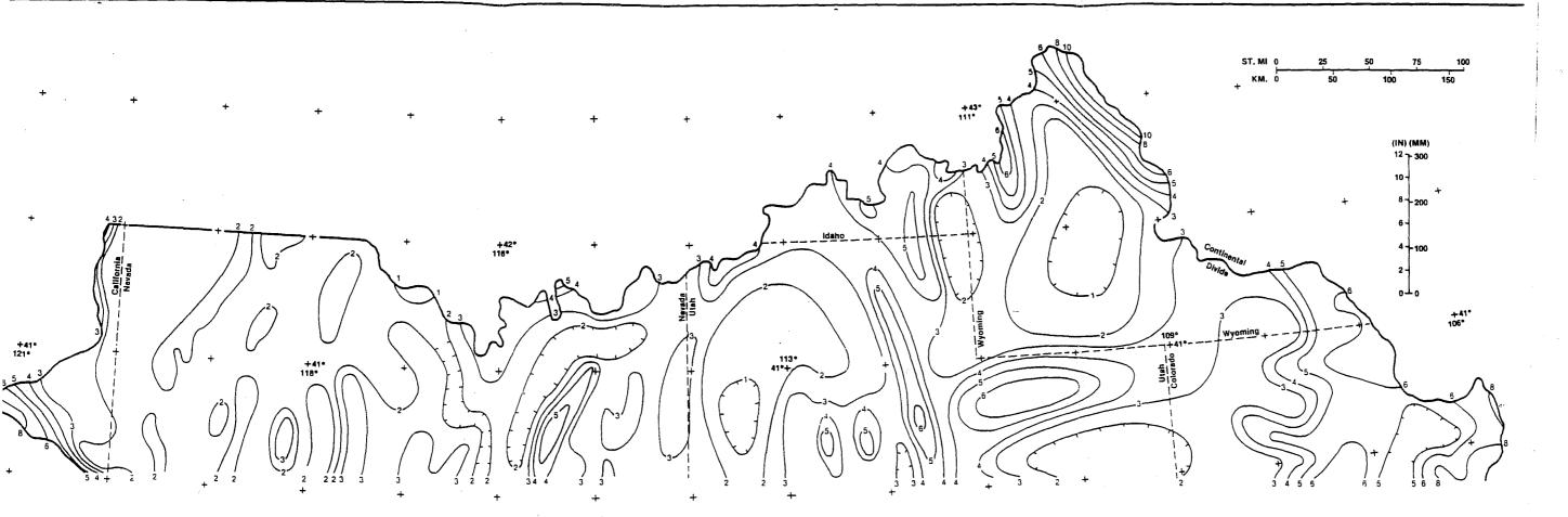
FIGURE 3.11a (Revised) — 10-mi² (26-km²) 24-hr orographic PMP index map (inches), northern section.
