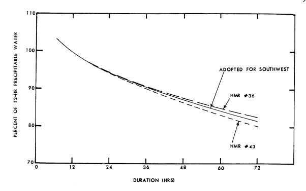
Figure 3.23. -- Durational variation of precipitable water.
