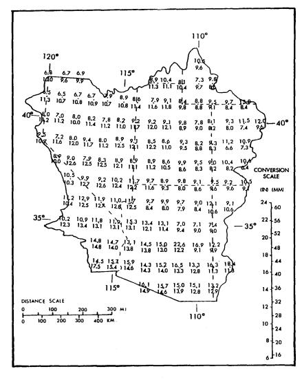
Figure 5.4.--General-storm PMP for 10 mi<sup>2</sup> (26 km<sup>2</sup>) 24 hr in inches (upper number) and local-storm PMP for 10 mi<sup>2</sup> (26 km<sup>2</sup>) 6 hr in inches (lower number) at 1° grid points.
