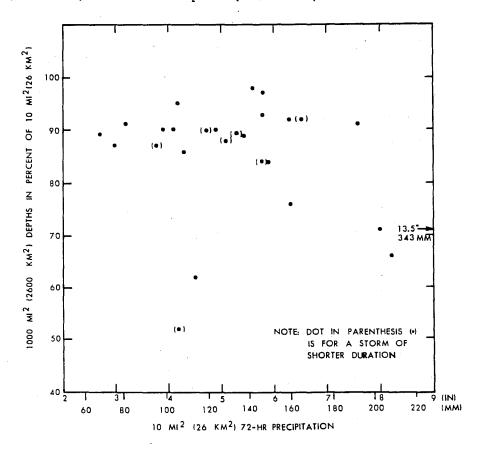
Figure 3.21.--1000-mi<sup>2</sup> (2590-km<sup>2</sup>) storm depths relative to 10-mi<sup>2</sup> (26-km<sup>2</sup>) depths for 72-hr rainfalls.
