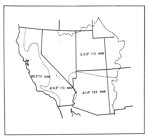
Figure 4.6.--Criteria of clock-hour rainfall amounts used for selection of storms at recorder stations for depth-duration analysis.
