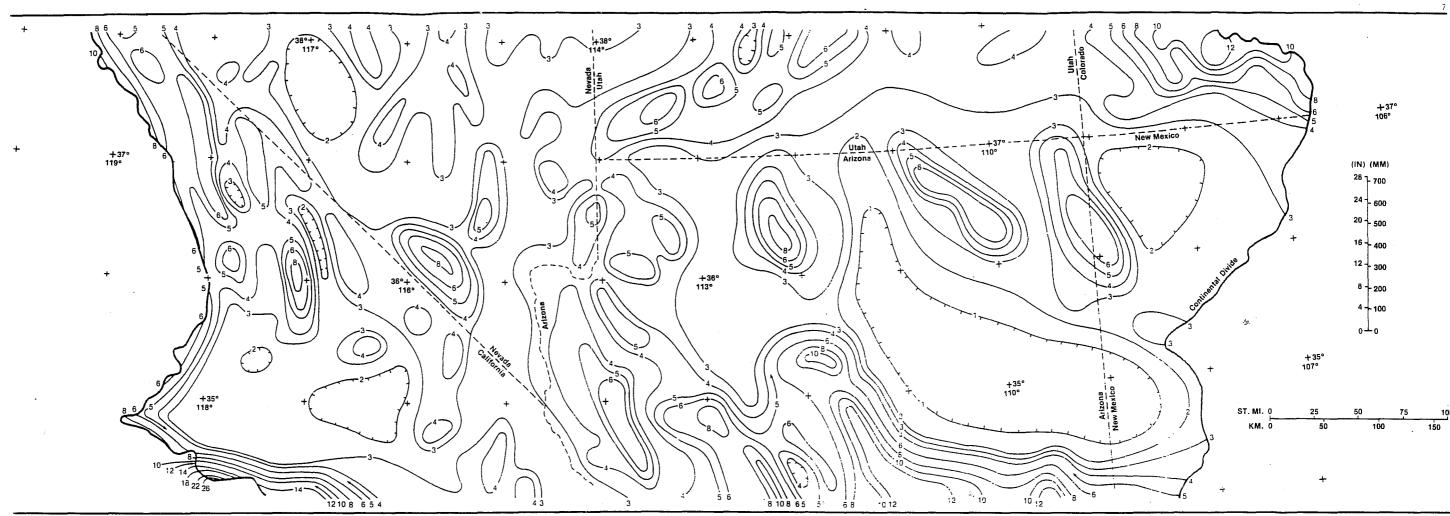
FIGURE 3.11c (Revised) — 10-mi² (26-km²) 24-hr orographic PMP index map (inches), south-central section
