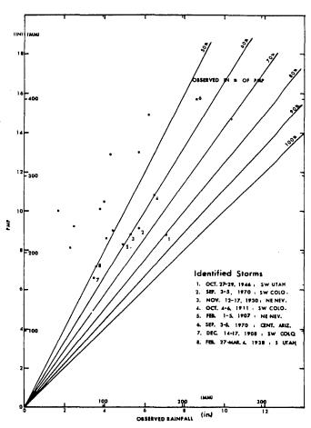
Figure 5.1.--Comparison between observed rainfall depths and general-storm PMP for 100 mi (259 km²) 24 hr.
