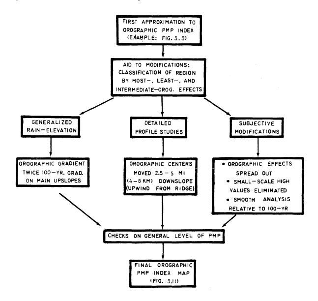
Figure 3.2. -- Schematic of orographic PMP index map development.
