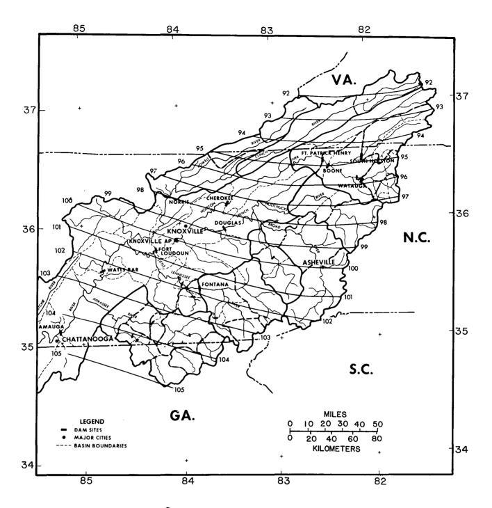
Figure 55.--24-hr 1,000-mi<sup>2</sup> PMP and TVA precipitation percentiles of Knoxville Airport for the eastern portion of Tennessee River watershed.
