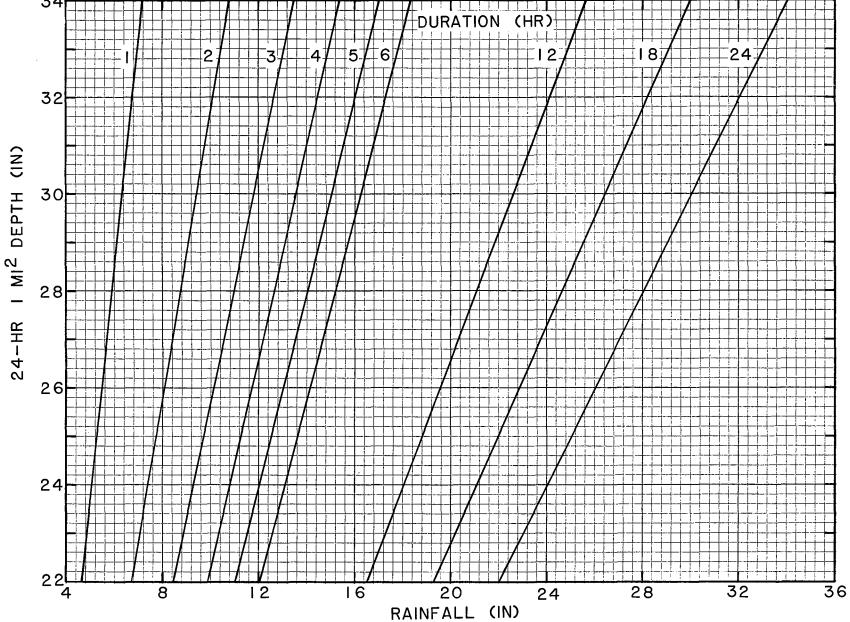
Figure 40.--Depth-duration relations for 24-hr TVA precipitation storm.
