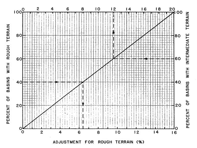
Figure 65.--Adjustments to large-area basins for terrain roughness valid for 100-mi<sup>2</sup> areas.
