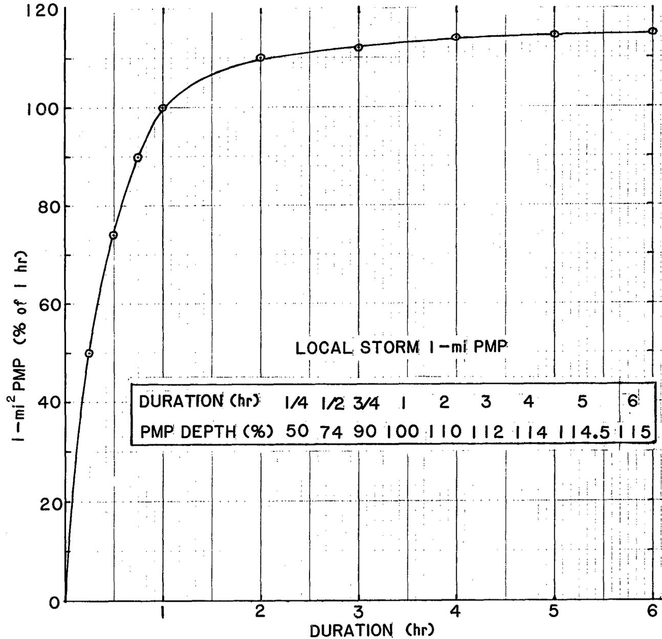
Figure 15.38.--Depth-duration relationship for 1-mi<sup>2</sup> PMP Pacific Northwest states (Section 11.7.2).
