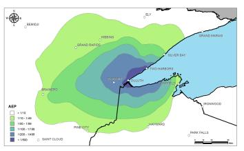
Example of a product occasionally produced by HDSC for extreme events, showing the severity of a rain event in terms of annual exceedance probability (AEP), the chance of rainfall equaling or exceeding a particular value. In this case, extreme rainfall in and around Duluth last May showed 24 hour rainfall with AEP more rare than 1 in 500.
