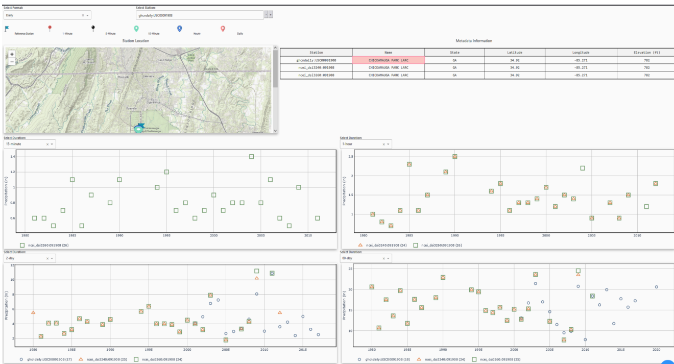
Figure 9. Co-located cleanup software, showing a location with a 15-minute, 1-hour, and 1-day timestep gauge, with varying periods of record and annual maxima.
