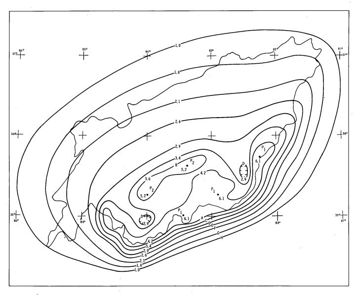
Figure 7-5. TVA March isohyets (21,400-sq. mi. upstream), 1st 6 hours
