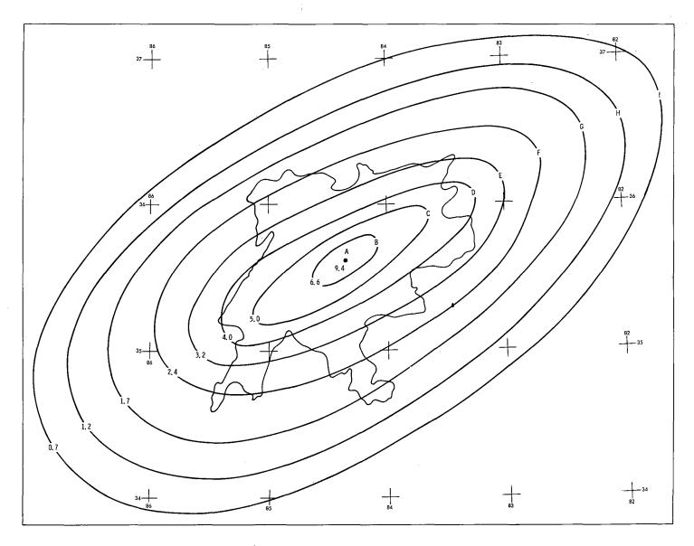
Figure 7-1. TVA March isohyets (7980 sq. mi.), 1st 6 hours
