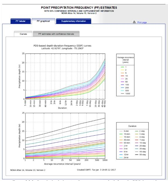
Figure 5.2.3. Sample depth-duration-frequency curves built from the PDS data with duration on the x-axis (top figure) and average recurrence interval on the x-axis (bottom figure).
