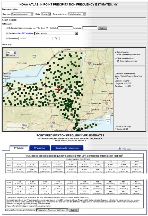
Figure 5.2.2. Initial view of the interactive map for the state of New York (when "Show stations on map" box is selected) with a data table under "PF tabular" tab.
