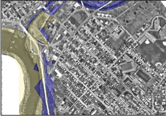
Figure 2 – Flood map comparing USGS data and AutoCAD data (1984 Flood).
