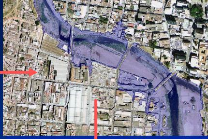
Water surface profiles are generated with HEC-RAS and can then be used for Flood Inundation Mapping
