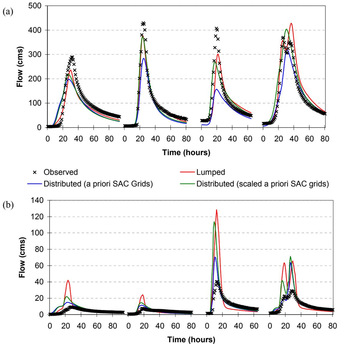
Figure 5. Simulations at (a) Eldon and (b) Peacheater Creek. Scaled parameters at Peacheater Creek are based on calibration at Eldon.
