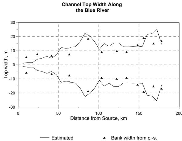
Figure 2. Comparison of estimated and observed top widths
