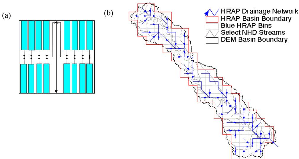
Figure 1. (a) Conceptual hillslopes and (b) cell-to-cell drainage network
