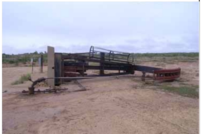
Pump jack turned over by tornado.
