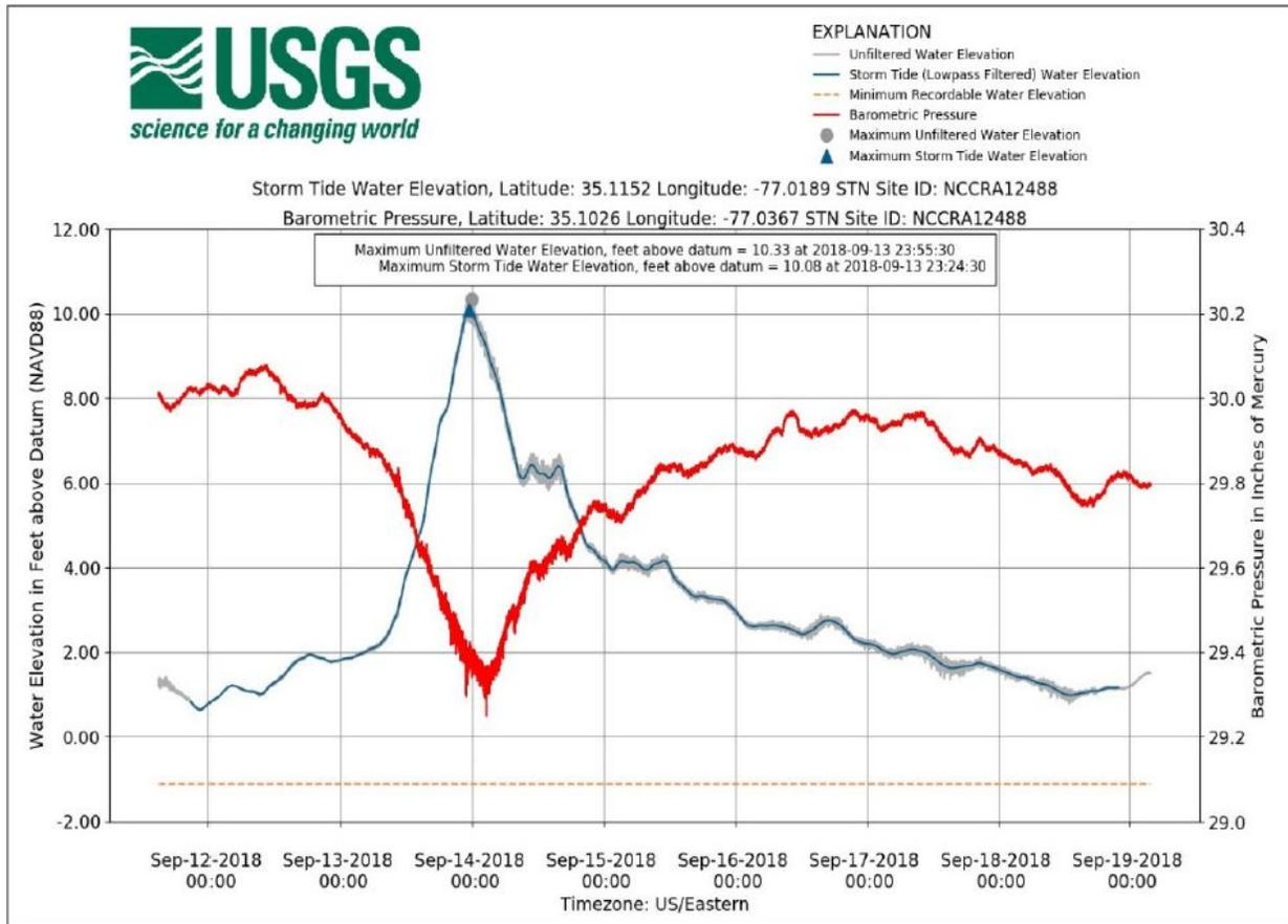
**Figure 4:** Instantaneous water level (gray, feet above NAVD88), wave-filtered water level (blue, feet above NAVD88) and barometric pressure (red, inches of mercury) recorded from a USGS sensor installed across the Neuse River from downtown New Bern, NC. Data were collected during the period September 11-19, 2018. *Source: USGS.*
