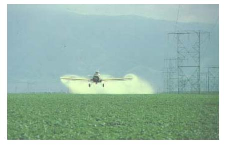
**Figure 2:** Thrush Commander applying fungicide spray on potatoes, southeast of Bakersfield, CA
