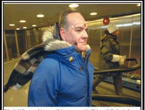
Wind chill test subjects walking on a treadmill in a chilled wind tunnel. Facial temperature readings were taken to help refine the new wind chill index.
