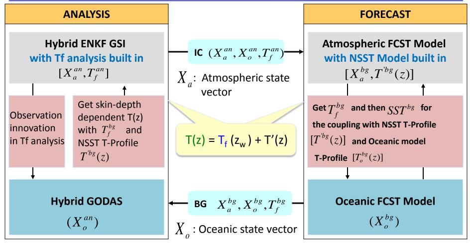
NSST algorithm is part of both the analysis and forecast system. In the analysis, the NSST provides an analysis of the the interfacial temperature ("SST") in the hybrid ENKF GSI using satellite radiances. In the forecast, the NSST provides the interfacial temperature (SST) in the free, coupled forecast instead of the temperature at 5-meter depth that is predicted by the ocean model.
