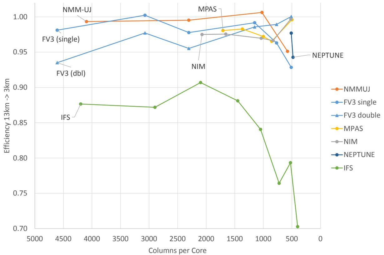
**Figure 7:** Weak scaling efficiency: the speed (grid-columns per second per core) running the 3 km workload divided by the speed running the 13 km workload for a given amount of work (grid-columns per core). In the case of NEPTUNE, there were only two overlapping core counts between the 13 km and 3 km benchmarks. (Higher is better metric; note that the scale of the Y-axis starts at 0.70, not zero.)
