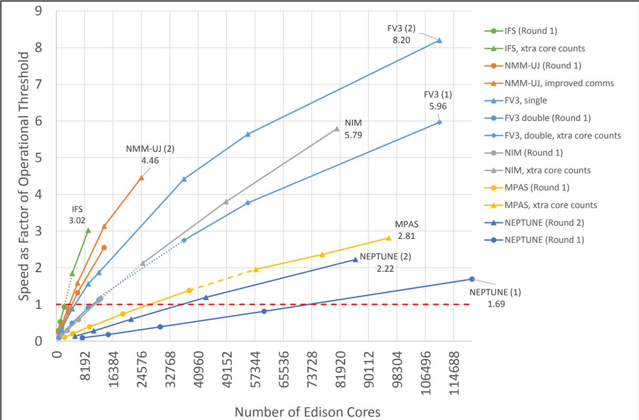
**Figure 3:** Speed as a function of number of cores, normalized to benchmark operational forecast integration rate of 8.5 min/day, shown as dotted red horizontal line at  $y=1.0$ . (13 km workload; higher is better metric.)
