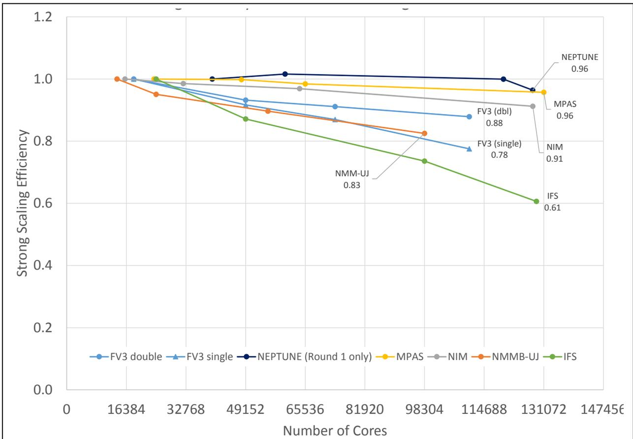
**Figure 6:** Strong scaling efficiency relative to fourth highest core counts. (3 km workload; higher is better metric.)
