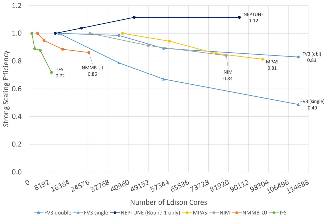
**Figure 4:** Strong scaling efficiency, defined as speedup relative to fourth highest core count divided by the increase in cores relative to fourth highest core count. (13 km workload; higher is better metric.)
