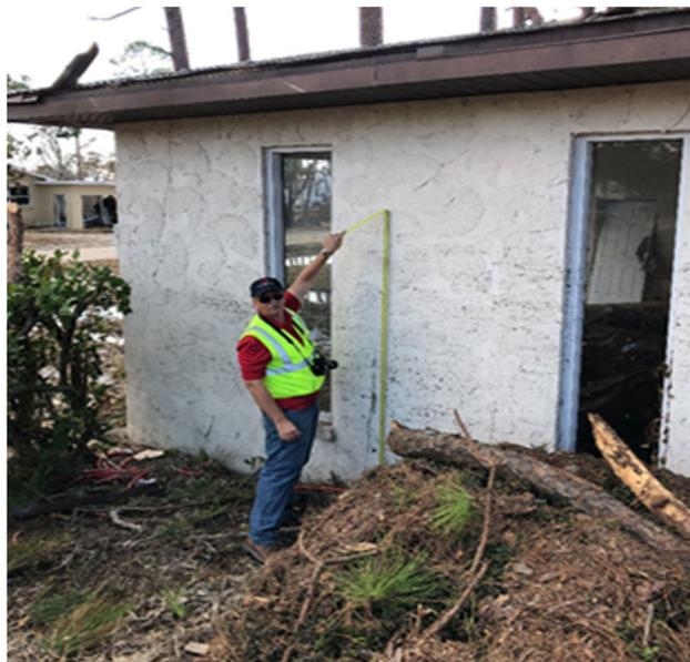
**Figure 36:** Surge high water mark (72") in Port St. Joe.
