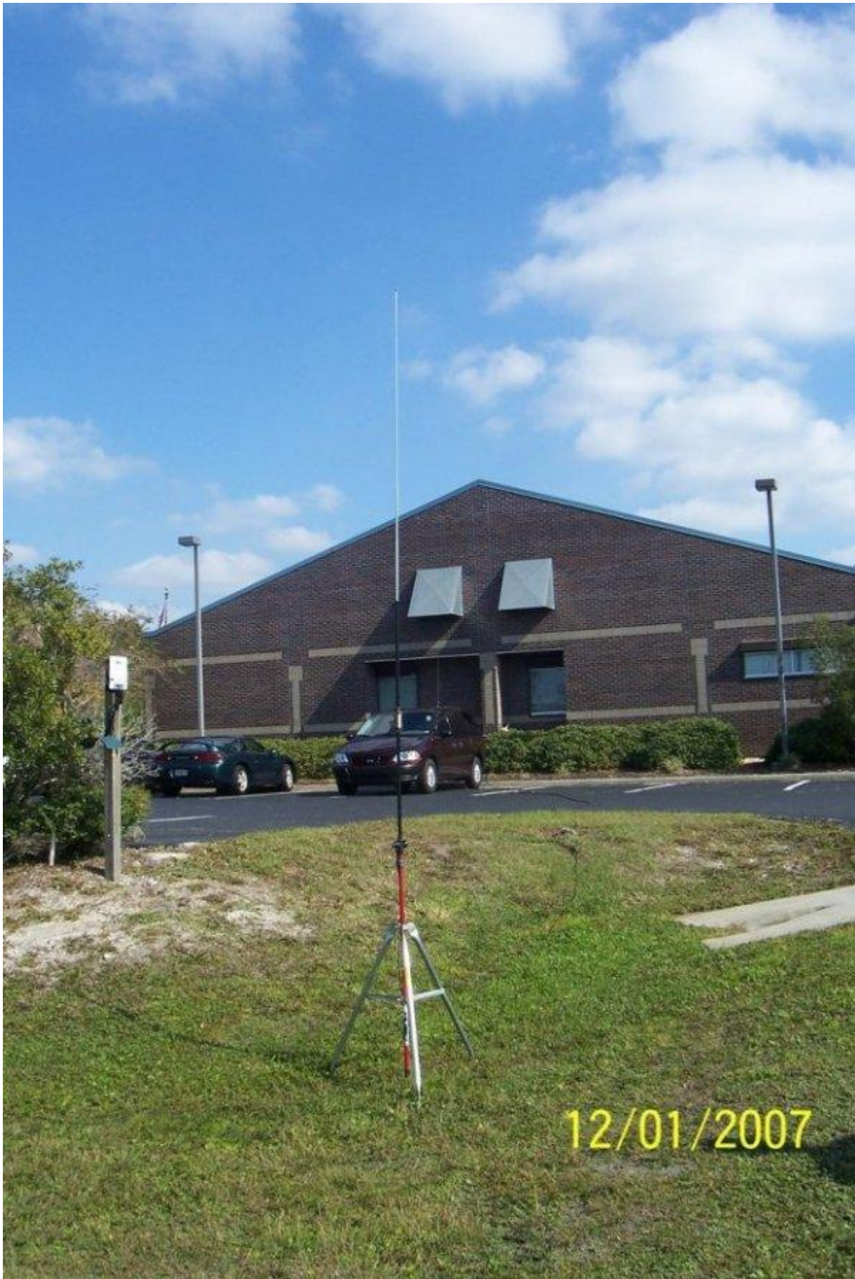
Numerous extra antennas were brought in and set up outside the WFO for this year's SRD. Antenna shown here is a Buddipole HF portable vertical antenna. Thanks to Ken Young, K1KEY, for providing the extra equipment
