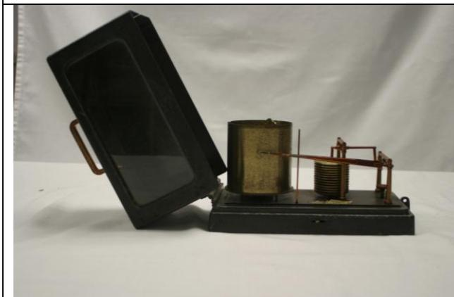
Barograph recorded a continuous stream of pressure onto graph paper.
