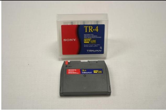
Sony TR-4 mini data cartridge storage tape that could hold up to four gigabytes of storage on a magnetic strip of tape.
