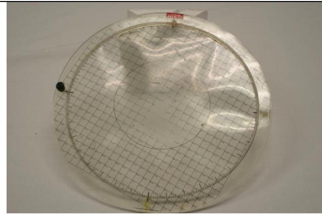
Manually digitized radar overlay for the WSR-57 radar. This was used to assign a video integrator and processor (VIP) level to each grid based on radar reflectivity. This data could then be used to later recreate a lower quality radar image.
