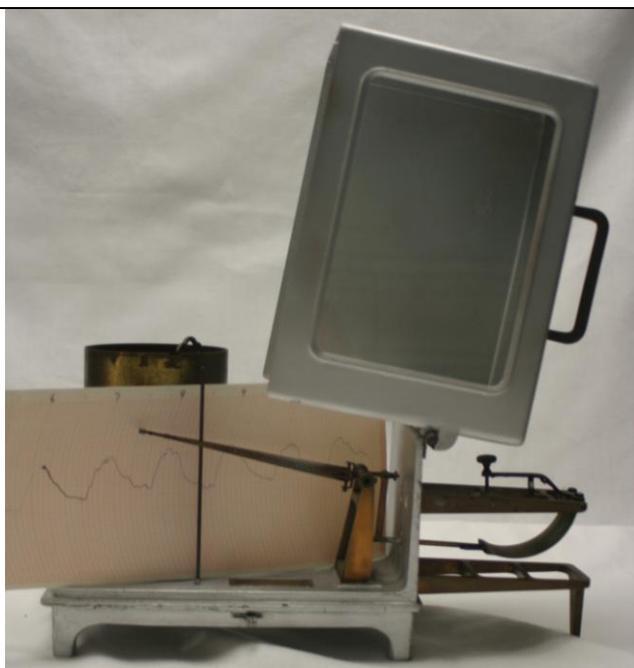
Thermograph which records temperature onto a continuously moving chart of graph paper.
