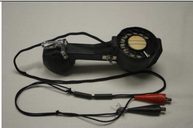
Electronic communication telephone handset with rotary dialer.
