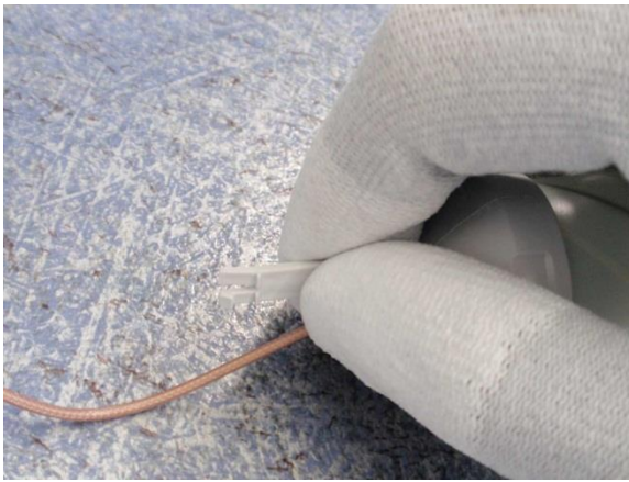
Exhibit F-9 Take a firm grip of the antenna's connection end
