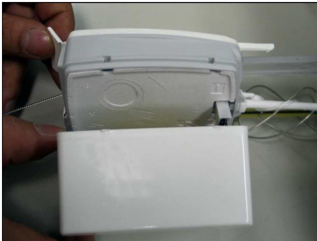
Exhibit F-13 Connecting the battery connector to the radiosonde
