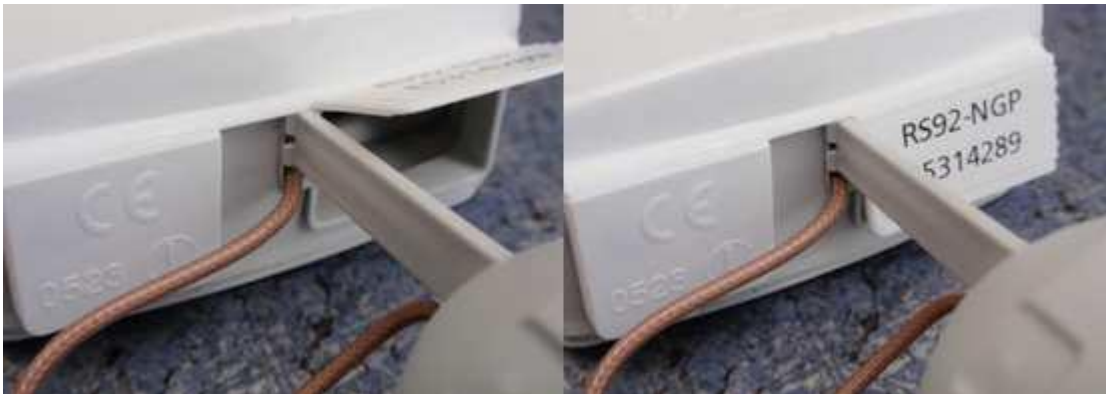
Exhibit F-10 Inserting the antenna clip into the opening
