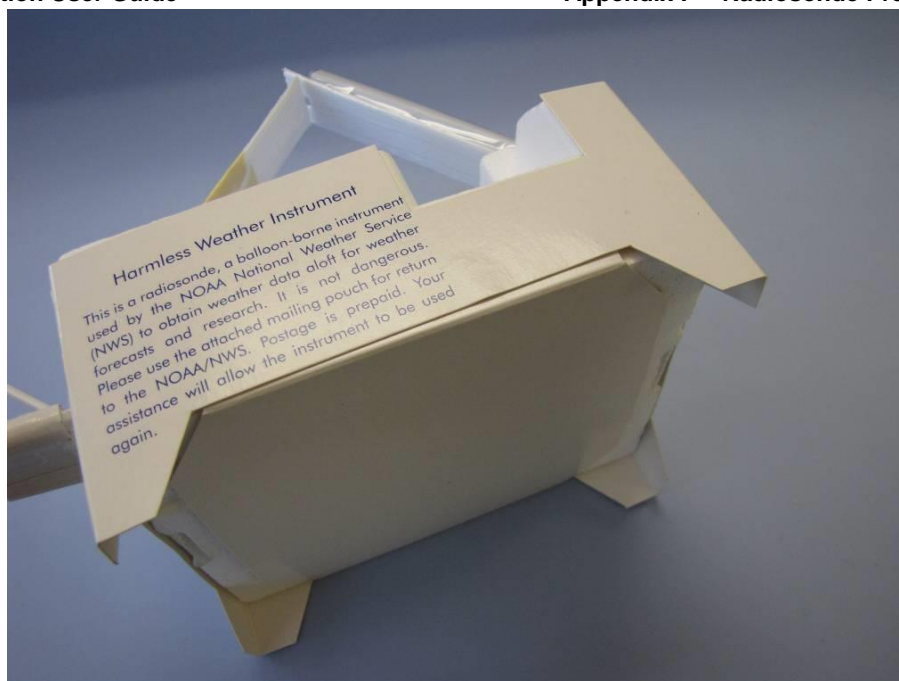
Figure 7 - Sealing the bottom of the sleeve.
