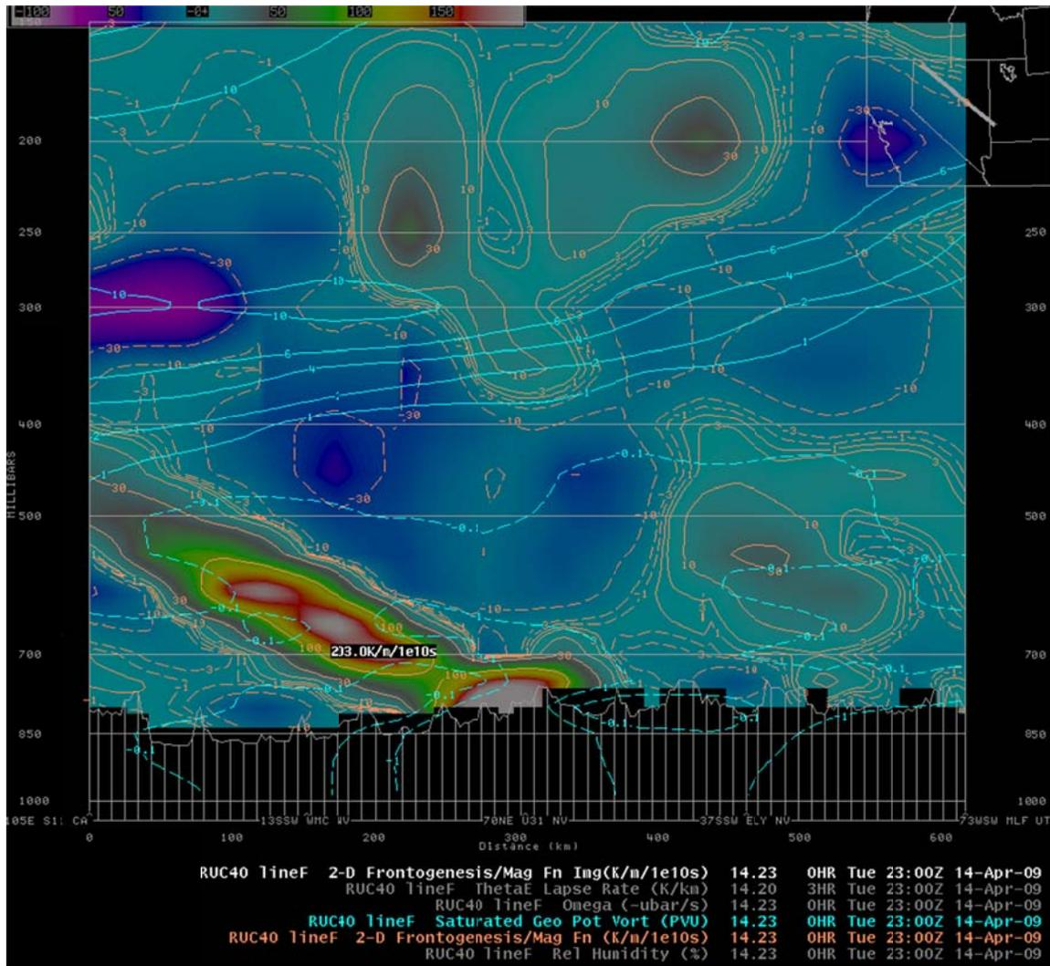
Figure 12: Same as Figure 11 except time is 2300 UTC. Note the frontogenetic forcing increased significantly in a three hour period.
