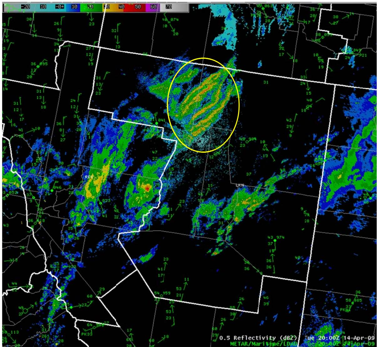
Figure 13: Composite radar (reflectivity) shows developing showers in east-central Nevada, 2000 UTC on 14 April. The banding seen in northern Nevada (yellow circle) was caused by chaff released from military aircraft.
