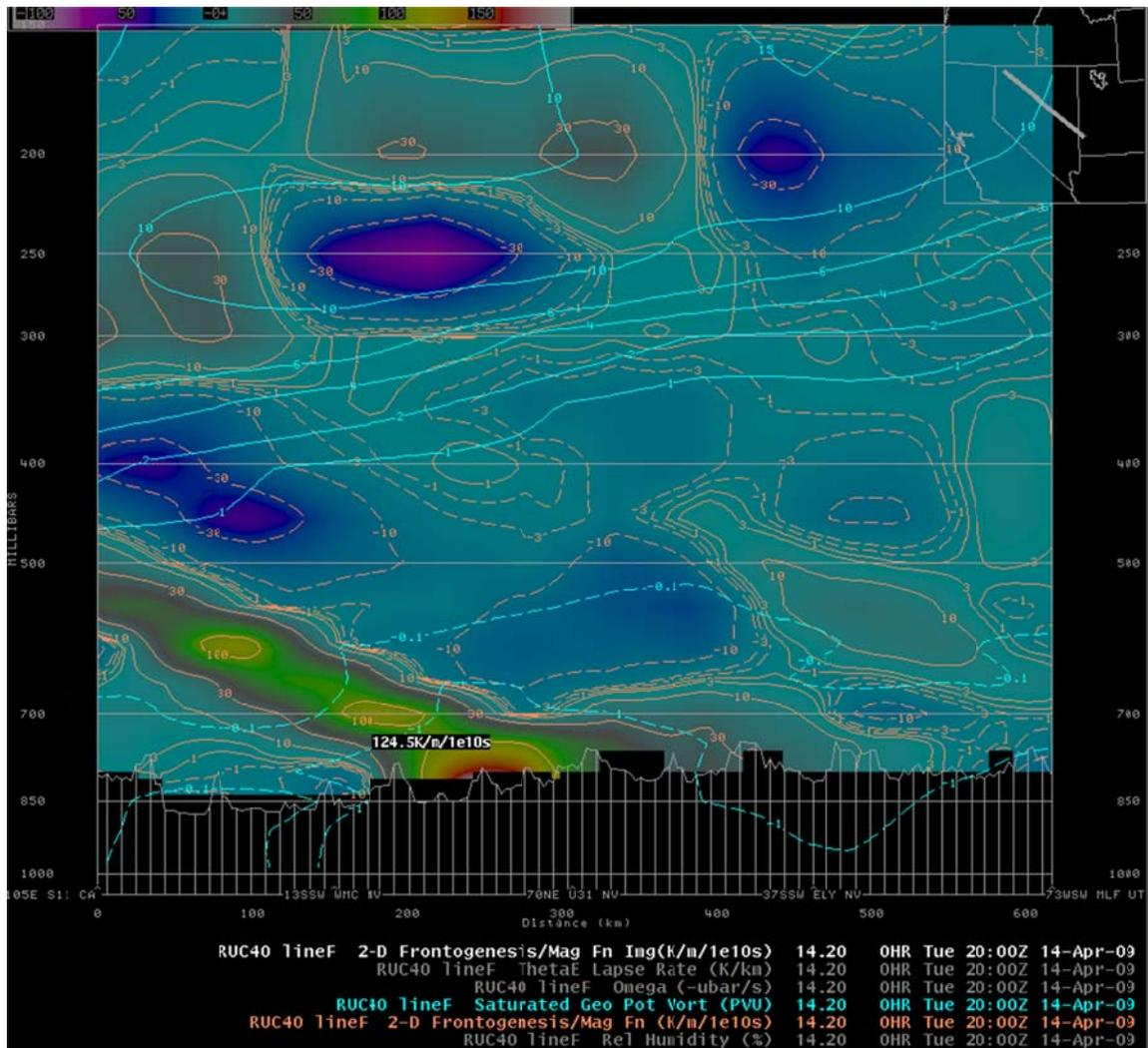
Figure 11: RUC40 00-hour analysis depicting cross section of Petterssen Frontogenesis (image, orange lines) with saturated equivalent potential vorticity (cyan lines, dashed lines are negative) for 2000 UTC 14 April. The area of maximum frontogenesis begins roughly 70 NM NE of Austin, NV (KU31) shifting west-northwest to 13 NM south-southwest of Winnemucca, NV (KWMC). The cross section extends from near Pioche, NV in the southeast to near Denio, NV in the northwest (see inset, upper right).
