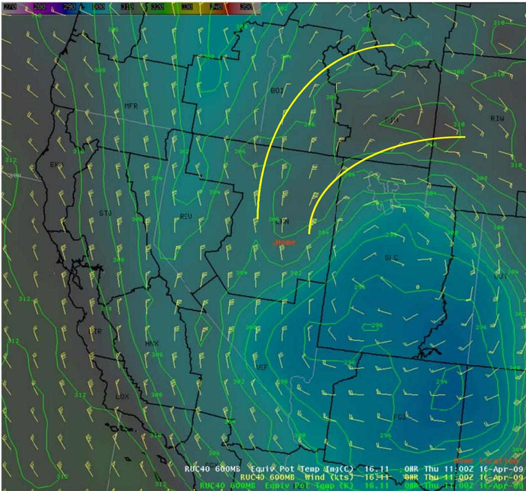
Figure 19: RUC40 analysis depicting 600 hPa equivalent potential temperature (green lines, solid) for 1100 UTC 16 April. Warmer colors indicate higher moisture values. “Home” position in red is positioned over Eureka, Nevada (KP68). Golden arcs depict the area of maximum equivalent potential temperature (trowel-like feature).
