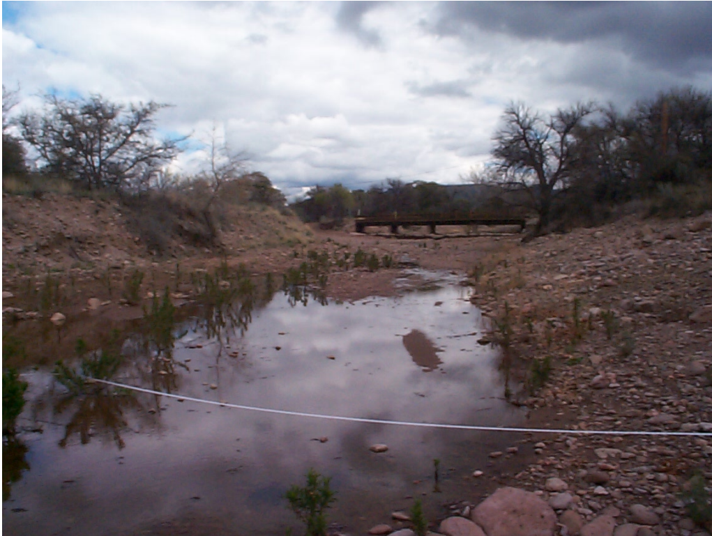
Figure 12: Cross section 1 looking upstream. Tape measure shows approximate position of cross section. Cross section 2 was located upstream near tree along right bank. Rucker Bridge and adjacent low water crossing seen in distance.
