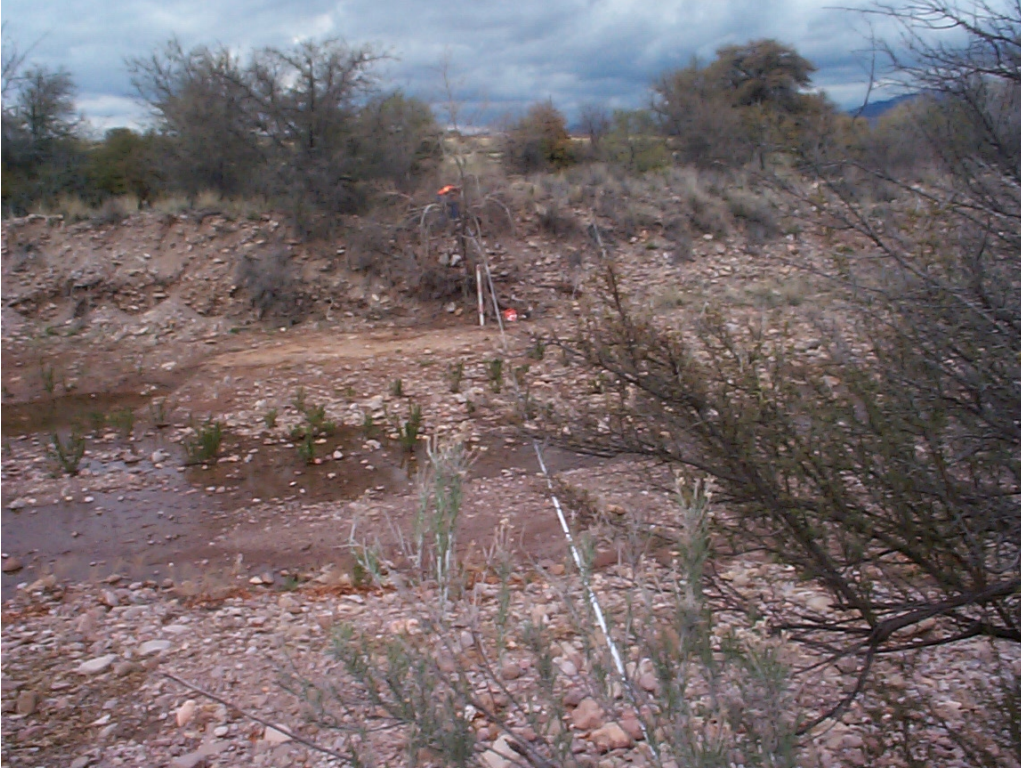
Figure 16: Cross section 2 as viewed from top of left bank looking north. Tape measure shows approximate position of cross section. High water mark located just above top of survey rod leaning against tree on right bank.
