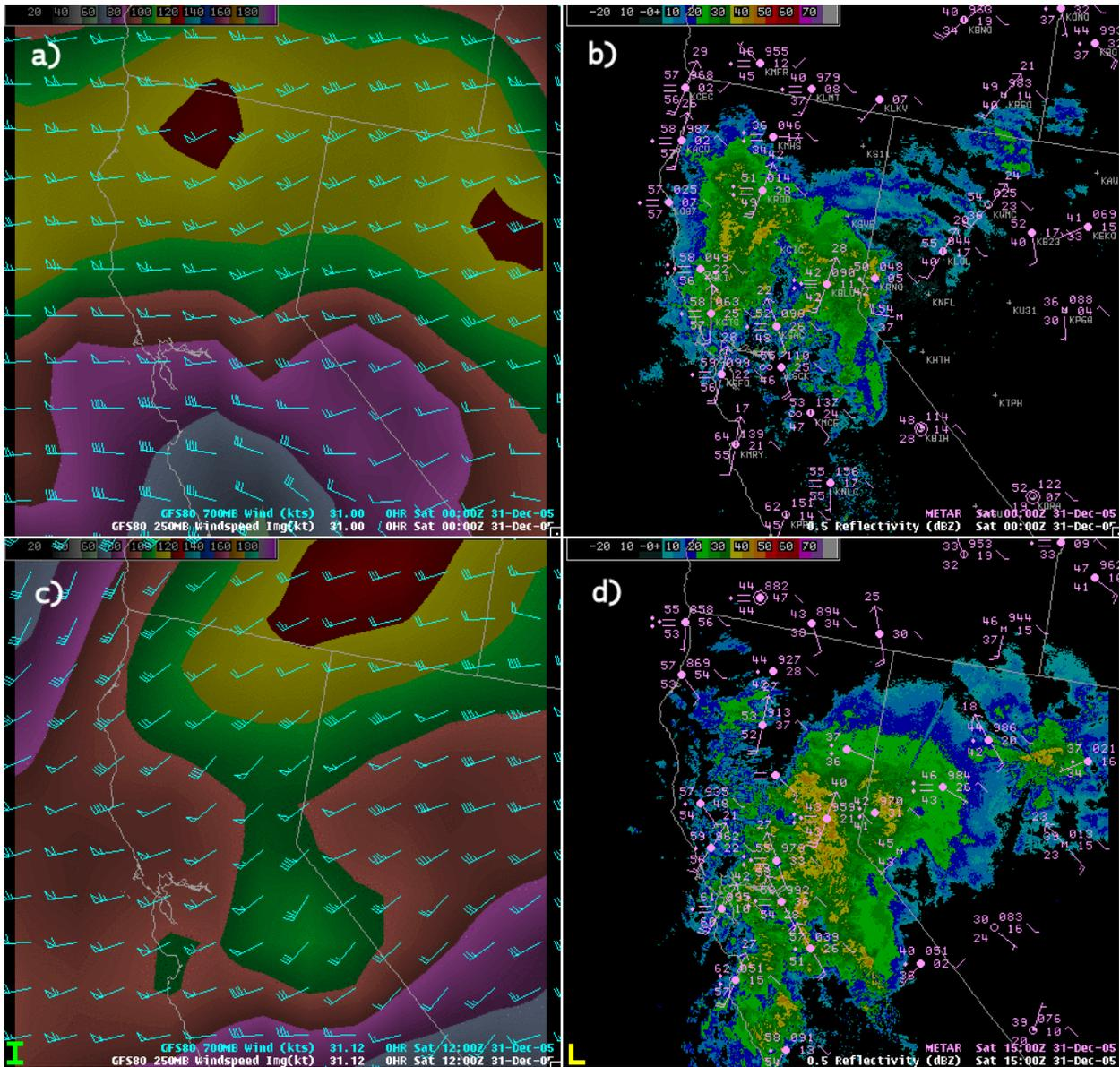
**Figure 3.** a) GFS analysis of 250 mb wind speed (shaded every 10 kts for with green shading indicating values between 100 and 110 kts) and 700 mb winds (barbs in kts) for 00 UTC 31 Dec 2005. b) 0.5 degree California-Nevada reflectivity mosaic and METAR plot at 00 UTC 31 Dec. c) Same as a) except the 12 UTC analysis. d) same as b) except at 15 UTC.
