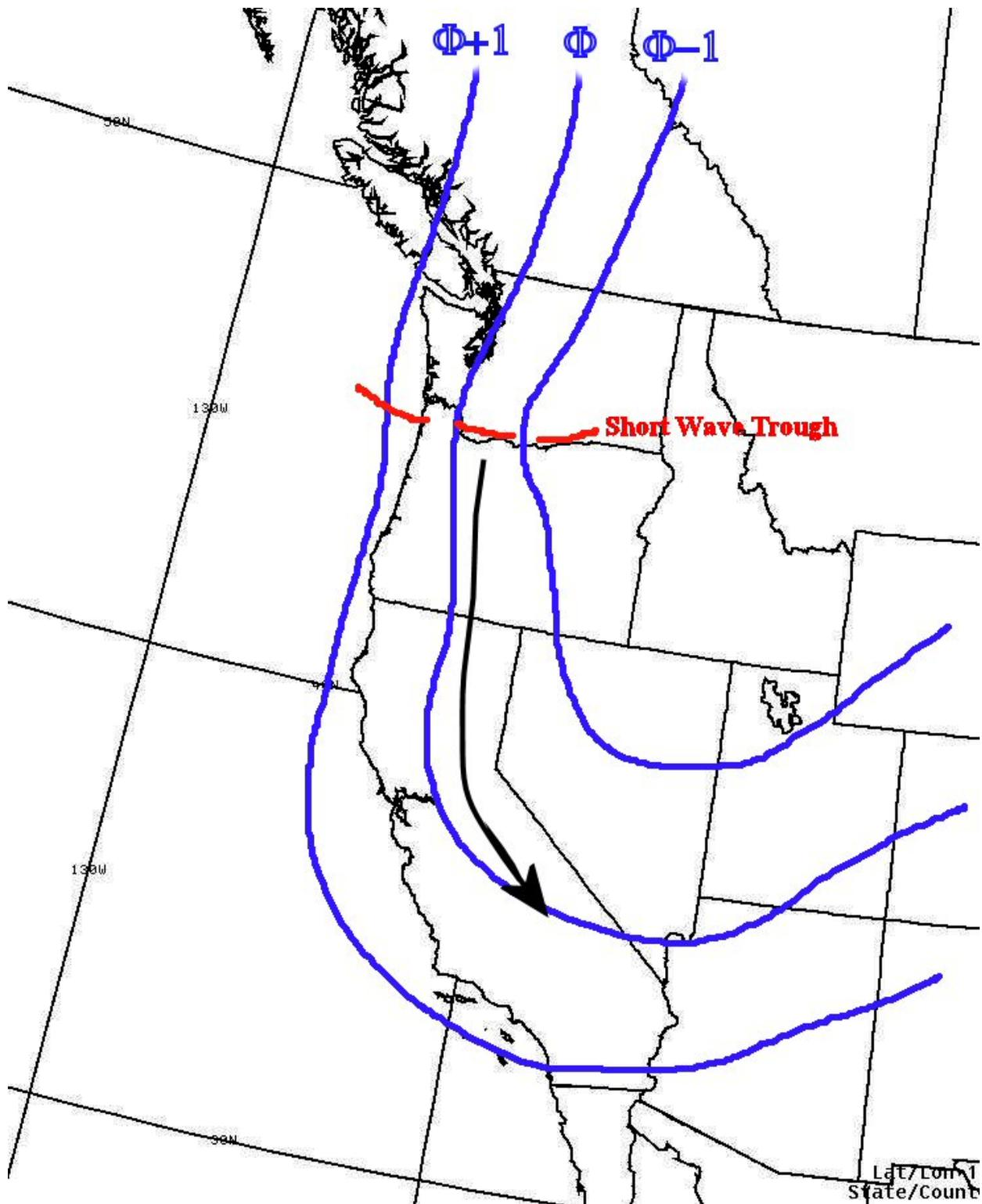
**Figure 12.** A 500 mb level schematic of the overall long wave trough across the Western United States, and the embedded short wave trough in the north-northwest flow on the upstream side of the long wave trough. Taken from Wallmann (2006).
