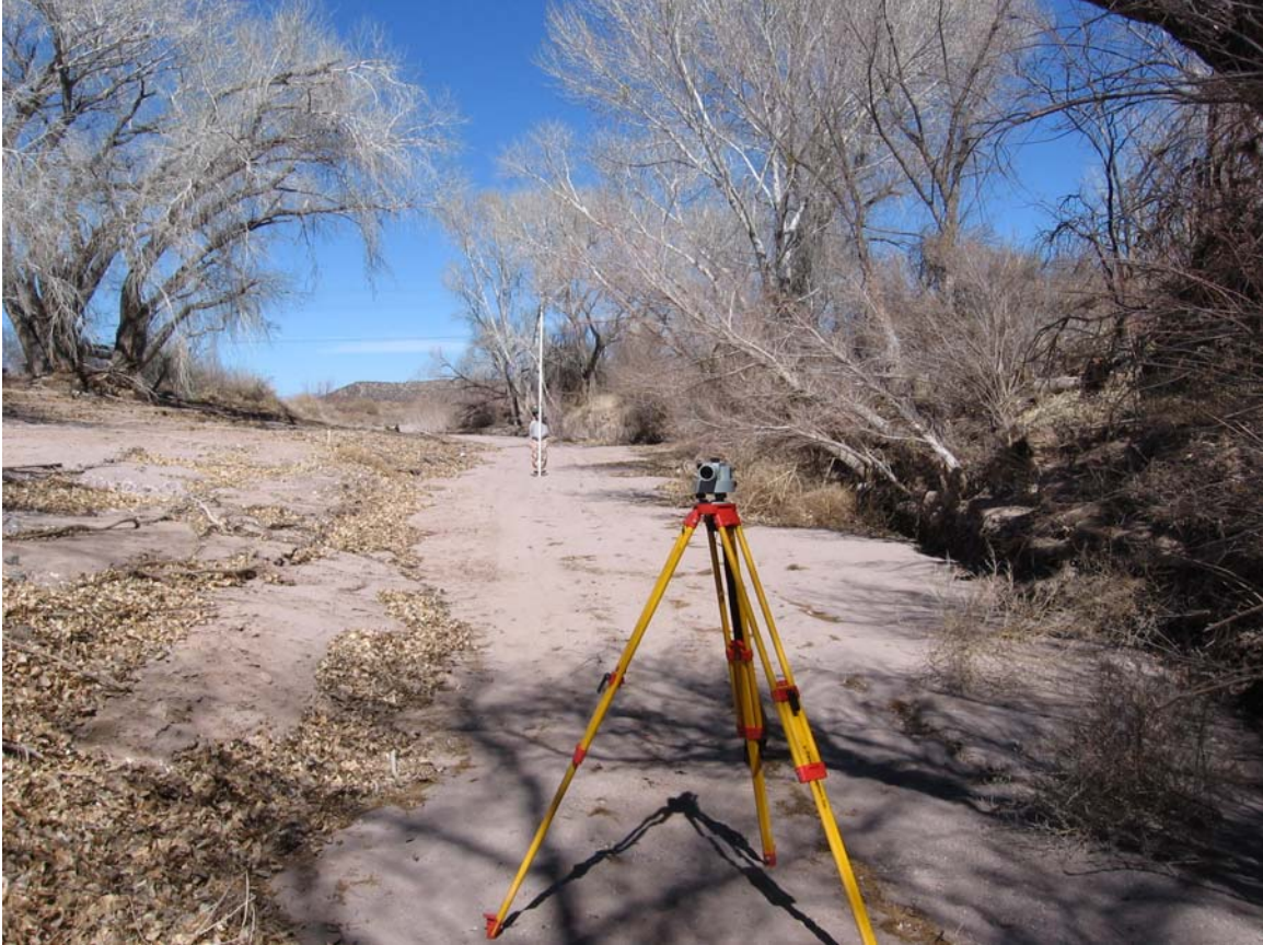
Figure 6: View looking downstream in low flow channel of Railroad Wash. Distance between cross sections was 100 feet, the same distance between the survey equipment as shown in the foreground and the survey rod in the distance. This was also the methodology used to determine channel slope.
