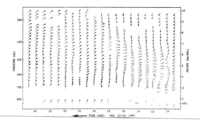
FIGURE 4. - This graphic represents a 24-hour history of 1-hour profile averages for one profiler site in northeastern Colorado. Note the passage of a low level disturbance between 10-122 and its reflection in the upper levels at later times.
