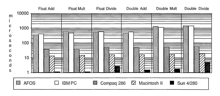
Figure 2: Benchmark execution time for each specified function on five different computers.
