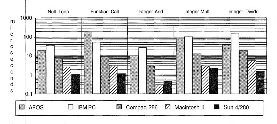
Figure 1: Benchmark execution time for each specified function on five different computers.
