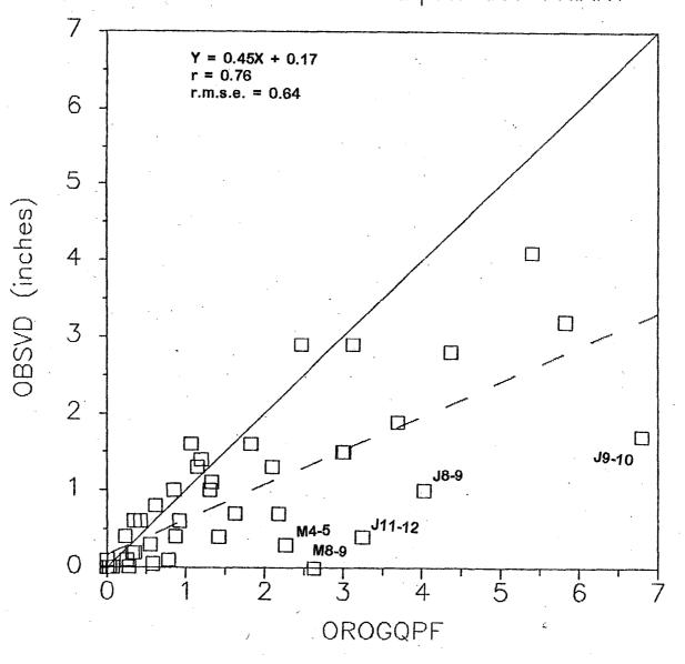
Figure 5. Predicted (X-axis) vs. Observed (Y-Axis) for San Joaquin River Basin above Friant Dam.
