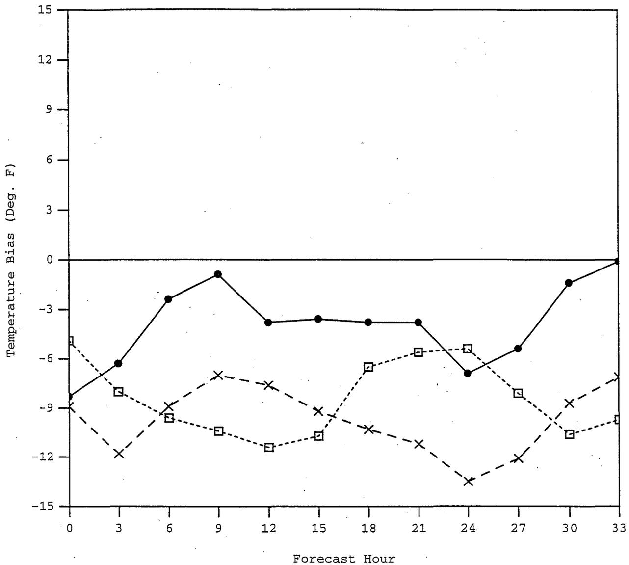
Fig. 1. Temperature bias ( $^{\circ}\text{F}$ ) for the 10-km Meso Eta 0300 UTC run (solid), the 29-km Meso Eta 0300 UTC run (dashed), and the 29-km Meso Eta 1500 UTC run (dotted) for the 0- to 33-h forecast periods covering early April through mid-August 1997.
