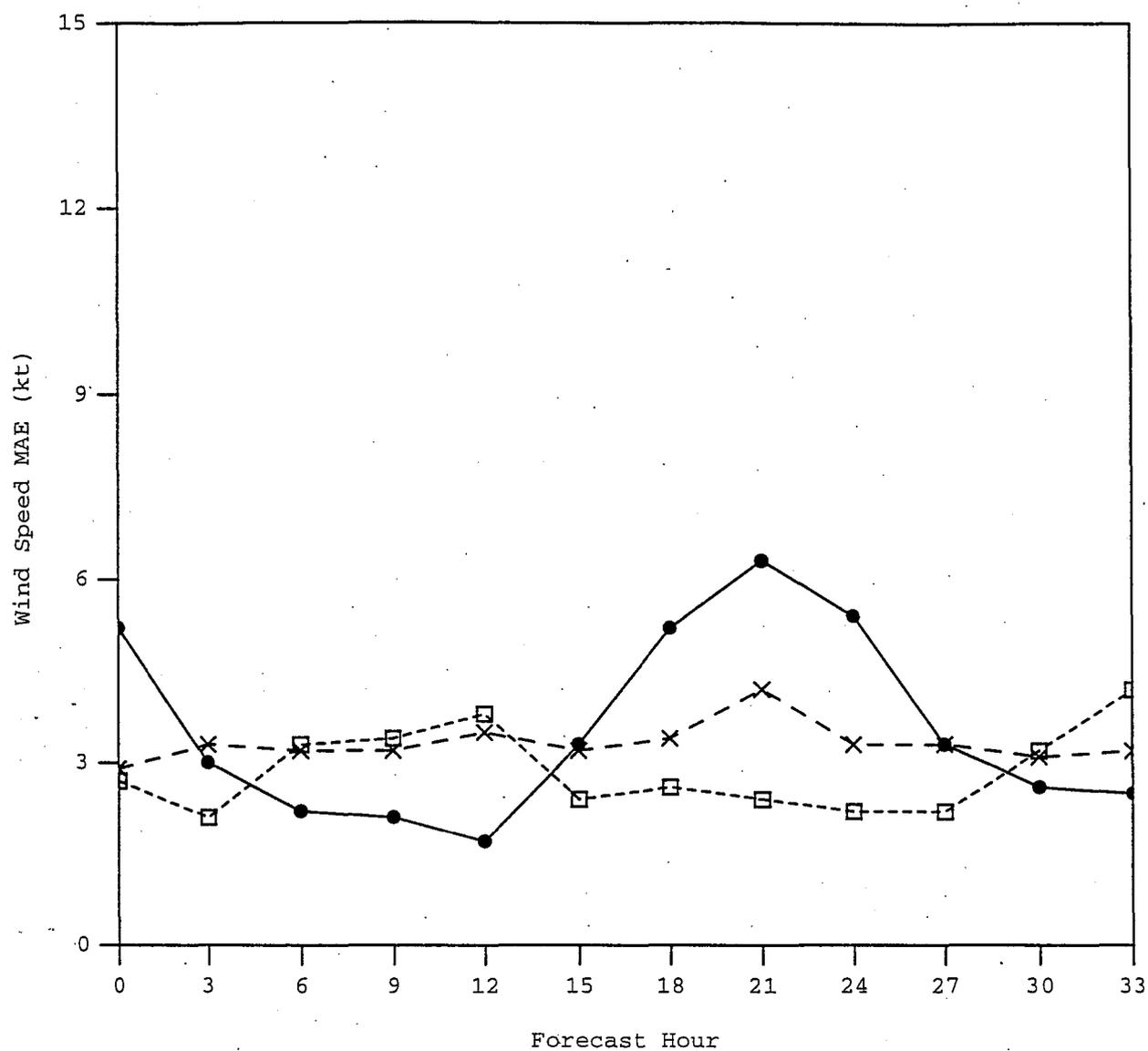
Fig. 6. Mean absolute error of wind speed ( $^{\circ}$ F) for the 10-km Meso Eta 0300 UTC run (solid), the 29-km Meso Eta 0300 UTC run (dashed), and the 29-km Meso Eta 1500 UTC run (dotted) for the 0- to 33-h forecast periods covering early April through mid-August 1997.
