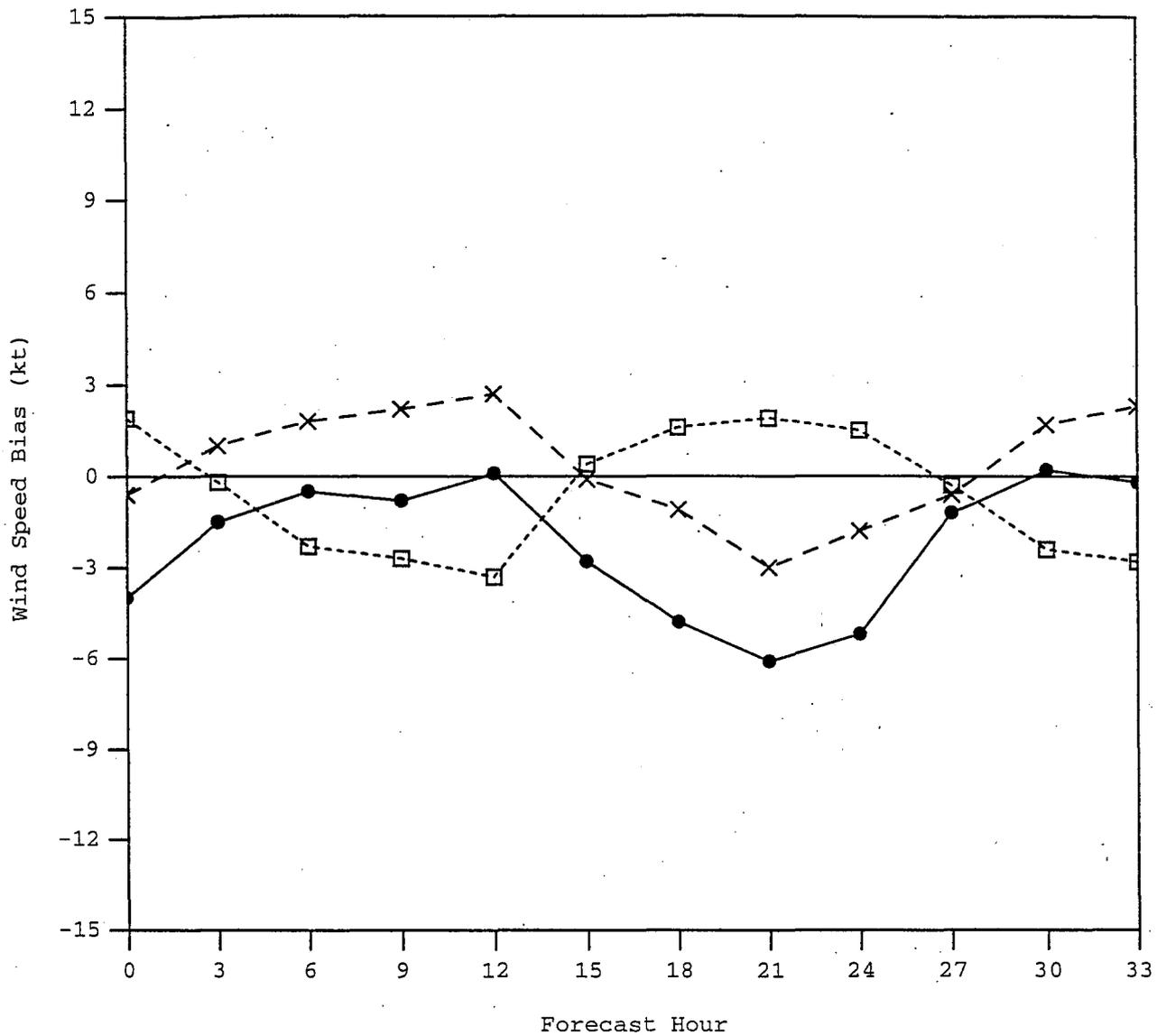
Fig. 5. Wind speed bias (kt) for the 10-km Meso Eta 0300 UTC run (solid), the 29-km Meso Eta 0300 UTC run (dashed), and the 29-km Meso Eta 1500 UTC run (dotted) for the 0- to 33-h forecast periods covering early April through mid-August 1997.
