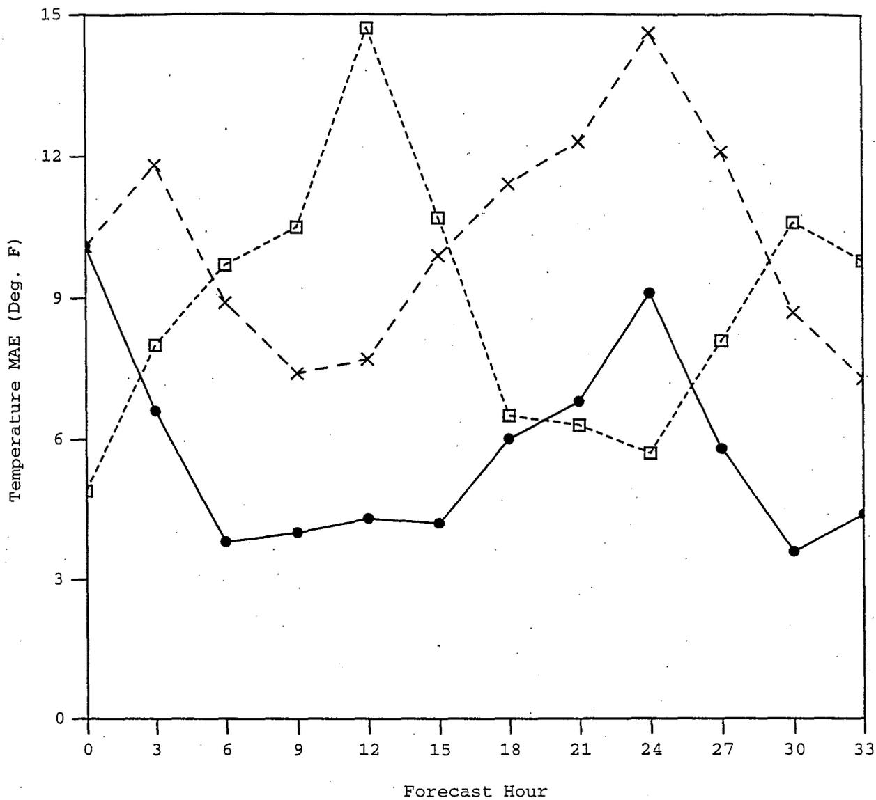
Fig. 2. Mean absolute error of temperature ( $^{\circ}$ F) for the 10-km Meso Eta 0300 UTC run (solid), the 29-km Meso Eta 0300 UTC run (dashed), and the 29-km Meso Eta 1500 UTC run (dotted) for the 0- to 33-h forecast periods covering early April through mid-August 1997.
