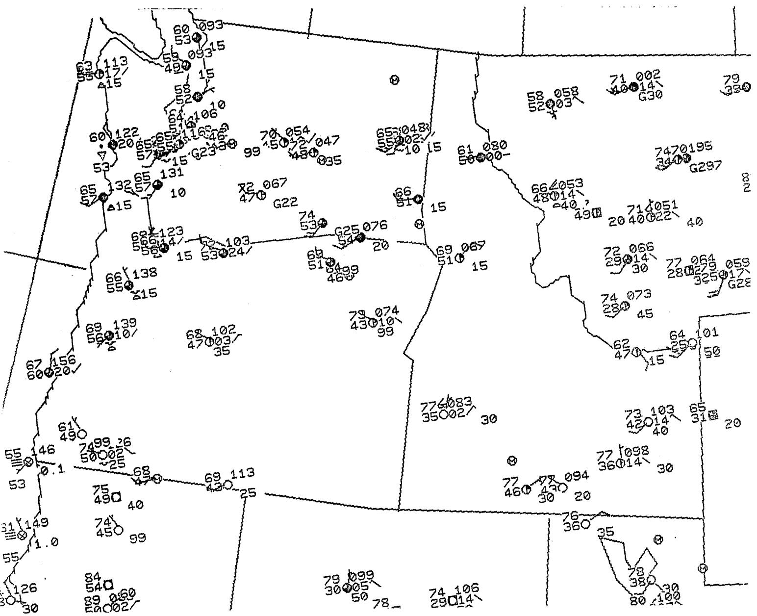
Figure 1: Surface Aviation Observation plot produced by the enhanced plotter. All parameters except visibility are in their correct locations. The comment field of the station model is used to plot precipitation, wind gusts, and visibility on a priority basis.
