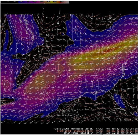
Figure 1 - GFS 00-hr analysis of 250mb winds at 12Z on December 17<sup>th</sup>. Isotachs are contoured every 10 knots. Note the core of strong winds of 120 knots or greater, indicative of a jetstreak, located across southern parts of California and Nevada extending into Arizona.
