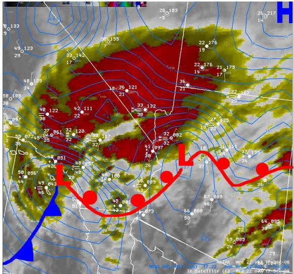
Figure 10 – Infrared satellite image with MSLP analysis (blue lines denote mean sea level pressure every 10 millibars) and plotted METAR observations at 22Z on December 17<sup>th</sup> with surface front analysis.
