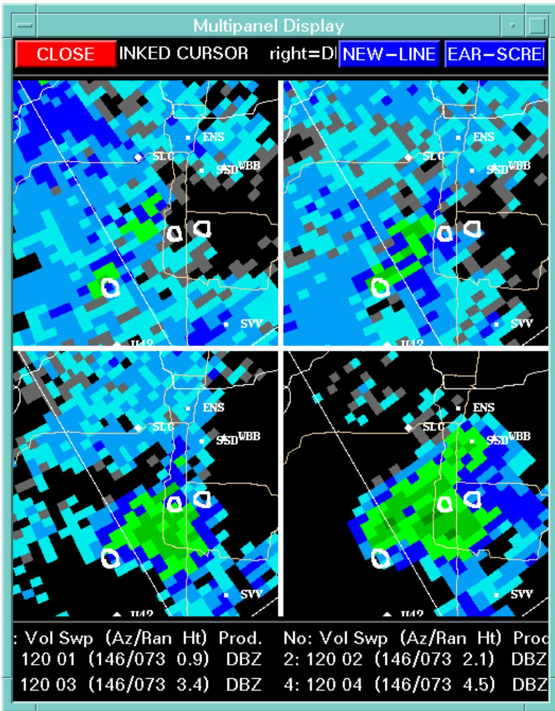
The velocity field at the 0.5 deg tilt (Fig. 6) shows a hint of divergence between SLC and U42 with 20 kts the maximum radial velocity, but nothing close to the 50+ kt winds reported at any of the three locations shown. Weak divergence at 0.5 deg gives way to 23 kts convergence at the 3.4 deg tilt.
