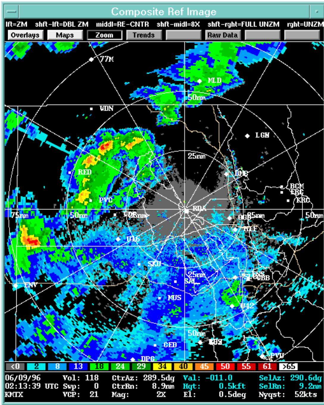
The peak reflectivity in the microburst storm occurred at 0144 (Fig. 2). The maximum reflectivity in the composite is 32 dBZ. However, there area greater than 30 dBZ (minimum threshold for cell ID algorithms) is not large enough to constitute a storm cell.
