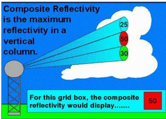
**Figure 6** – Diagram showing how composite reflectivity images are created by NEXRAD.
